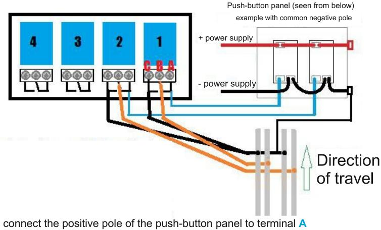
Connect the positive pole of the push-button panel to terminal **B** (optional) To have maximum braking when the power supply is disconnected, connect the negative pole of the lane of the track to terminal **C**
